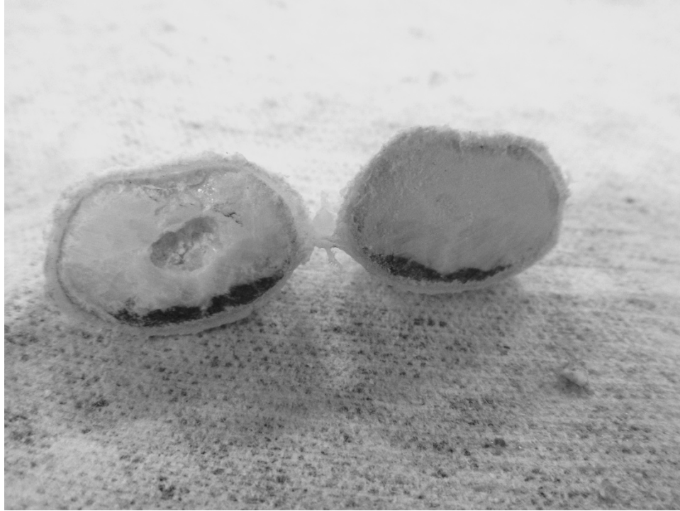
Figure 34 Bisected pellet containing sodium nitrate and 2 wt % NiO nanoparticles. The NiO is seen as the black material at the bottom of the pellet.
